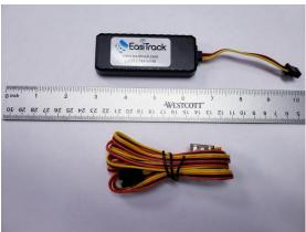
**Step 2)** Locate the constant 12 Volt Power Source, ignition and ground connections. Our GPS is shipped with a power harness, which has a 2 amp fuse attached. Possible sources for power harness installation are the main fuse block panel or the point where the vehicle charging circuit are connected to the 12 volt system.
